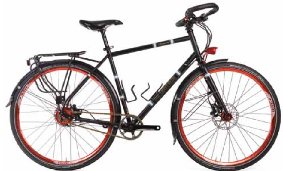
Speedtour bike shown is a custom version with added dynamo, mudguards and rack.
